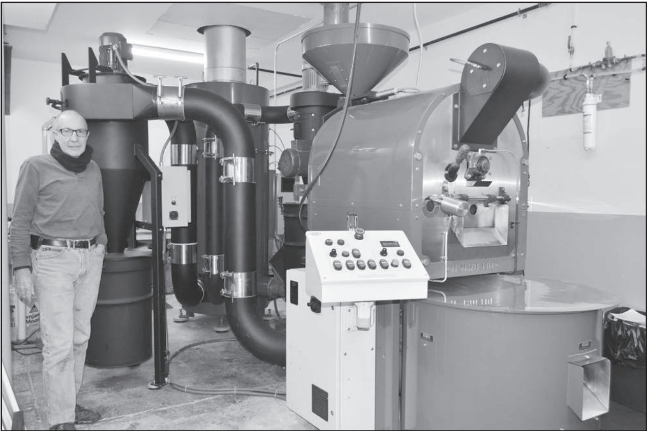
Eddie Giunta of Café Monte Alto was pleased to display the new baffling system installed on his coffee roasting oven that now keeps pollutants out of the atmosphere in downtown Plymouth.
