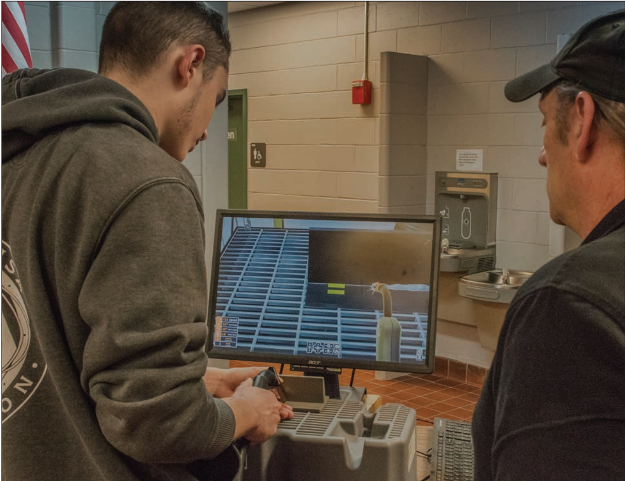
A STUDENT returned to the welding simulator to try to improve his technical score under the watchful eye of Collision Repair teacher Gary Sullivan. The simulator scores multiple factors as a person welds, says Sullivan, providing practice and feedback without the repeated expense of the metals and energy involved in actual welding.
