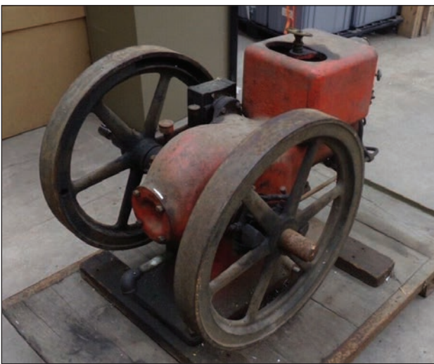
COURTESY This McCormick Deering hit-or-miss engine, typical of engines with large, heavy flywheels that could power all sorts of contraptions and run all day on a gallon of gas, was used as an all-around farm engine in Pennsylvania. It was for sale on ebay for $799. (Courtesy ebay)
