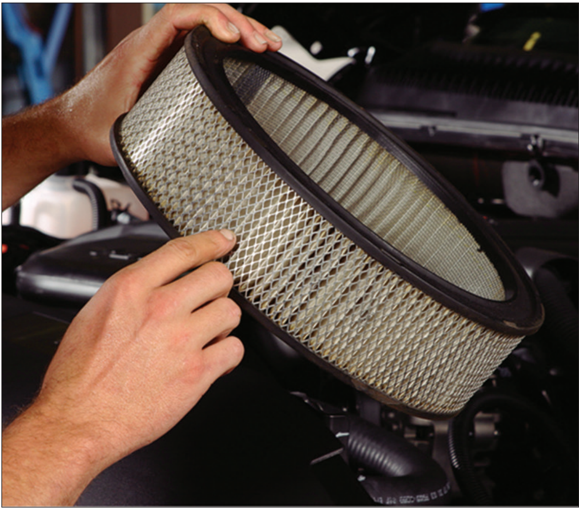
Replacing air filters is an inexpensive way to keep vehicles performing at peak capacity.
