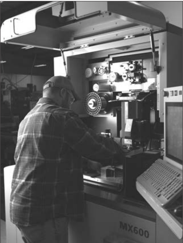
Seamus Quinlivan, machine operator, working with the Mitsubishi MX600 oil wire EDM machine at MTD Micro Molding.
