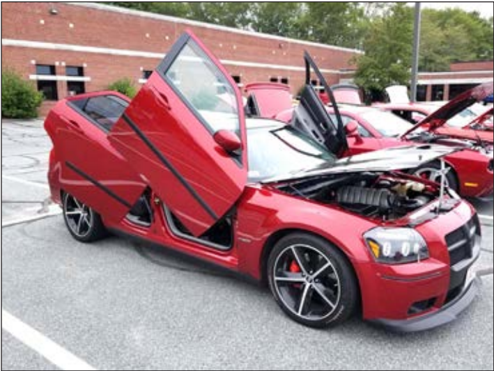
Butterfly doors aren't just for sports cars. This 2006 Dodge Magnum had all four doors converted
