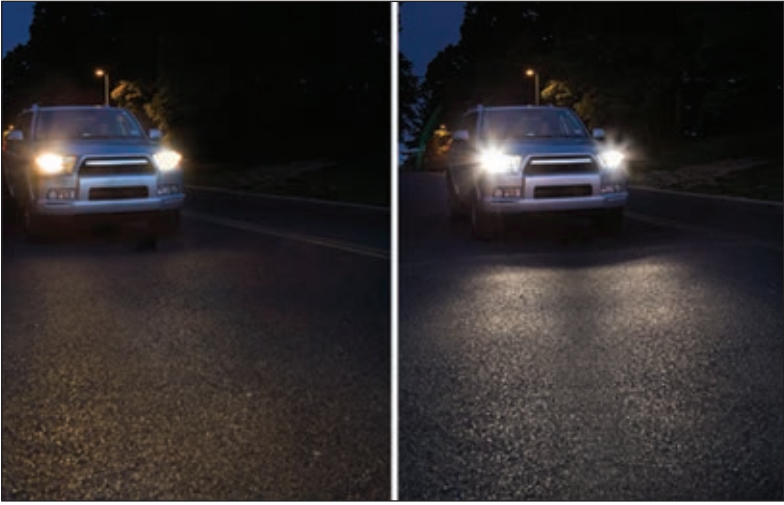
Philips Upgrade headlight bulbs (right) put more light on the road than older, more traditional halogen headlights, which are standard in many vehicles.
