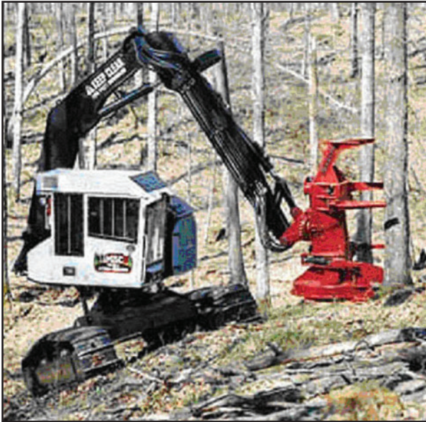
This is a feller-buncher, the tank-like treaded rig that has almost, but not quite, replaced the logger. Thanks to the region’s steep terrain, smaller land parcels, and rugged individualists who feel safer working alone, there are still a few cable-skidder loggers around the state.
